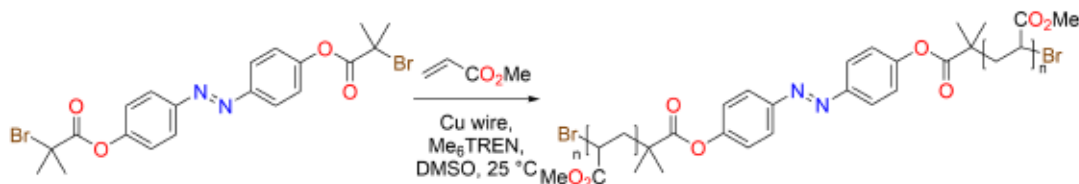
Scheme 1.9. SARA ATRP of methyl acrylate with a difunctional azobenzene-based initiator to diazocine-centered PMA. [19]
