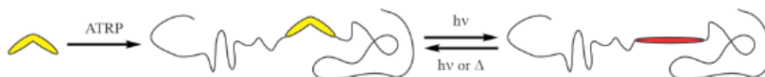
Scheme 2.2. Diazocine as an ATRP initiator to build diazocine-centered elastomeric chains. Yellow shape: ( Z ) diazocine. Red shape: ( E ) diazocine.
