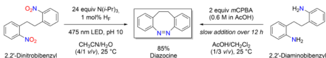
Scheme 1.5. N–N coupling of 2,2'-dinitro- and 2,2'-diaminobibenzyl under optimized reaction conditions. [75,76] H F : dye-infused Co-based metal-coordination cage.
